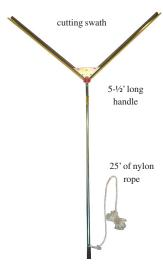
The Weed Razer is a lightweight, hand operated, underwater weed cutter. Available in 3 cutting swath sizes; 30", 48" and 9" to 62". Designed for easy use by a single person. Two angled stainless steel blades cut cleanly through weeds. Non-blade parts are zinc plated for corrosion resistance. Includes 25' of nylon rope and complete instructions.
